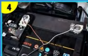
4 Wiring method A: Connect to battery power directly with the supplied power cable.
